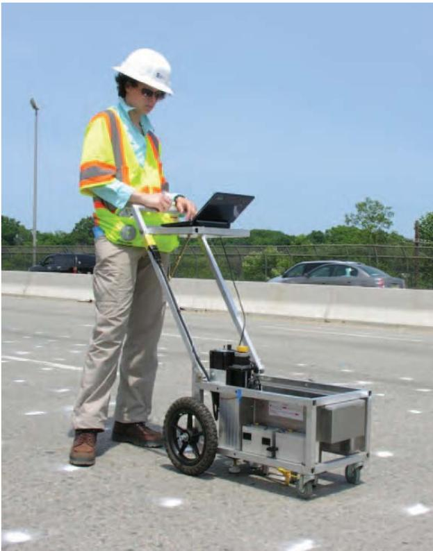
**Figure 07: PSPA Data Acquisition on the Bridge Deck with 2×2 feet Grid Spacing [18].**
