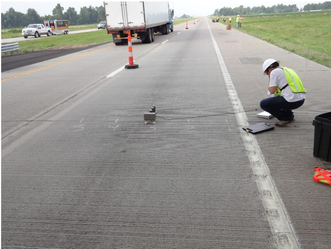
Figure 18: The PSPA In-situ Testing on Pavement Section 05.
